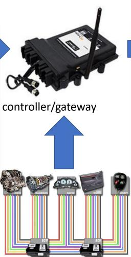
CANBUS; vehicle control and monitoring system
